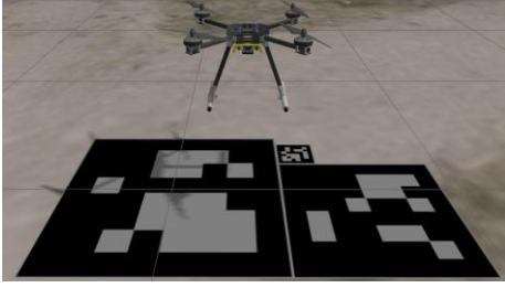
Fig. 1. Drone model with a cascade of ArUco markers in the Gazebo simulator
