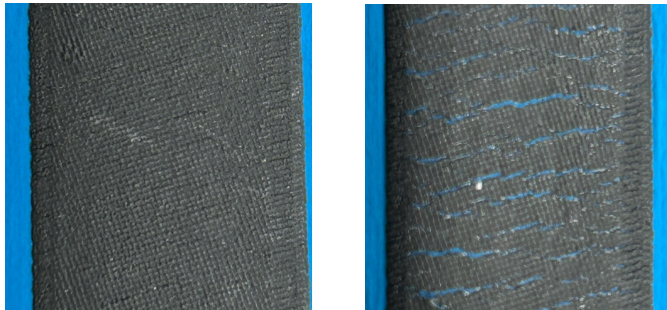
Fig. 4. Silver-carbon layer before (left) and after (right) 25 % elongation
