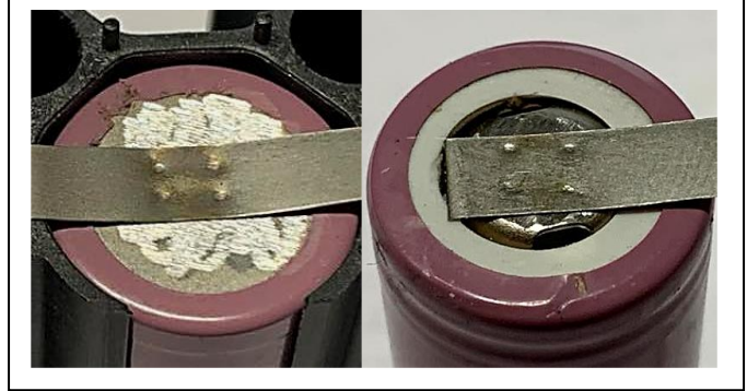
Fig. 10. Spot-welded connections on cylindrical cells of size 18650, maximum power output on the left, and low power output on the right.
