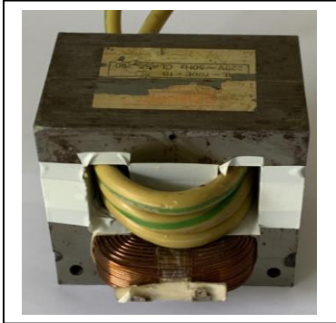
Fig. 5. The custom power transformer modified for high current output.
