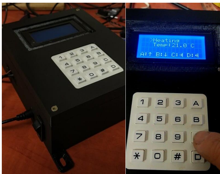
Figure 3: Aquarium control system in box with user interface and program menu
