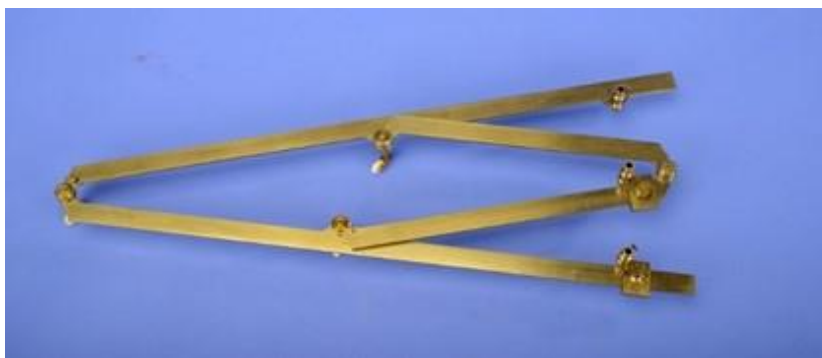
Figure 1: Example of pantographic mechanism [1]
