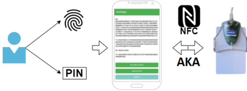
Figure 1: Multi-factor authentication system using smart phone and embedded SAM module.
