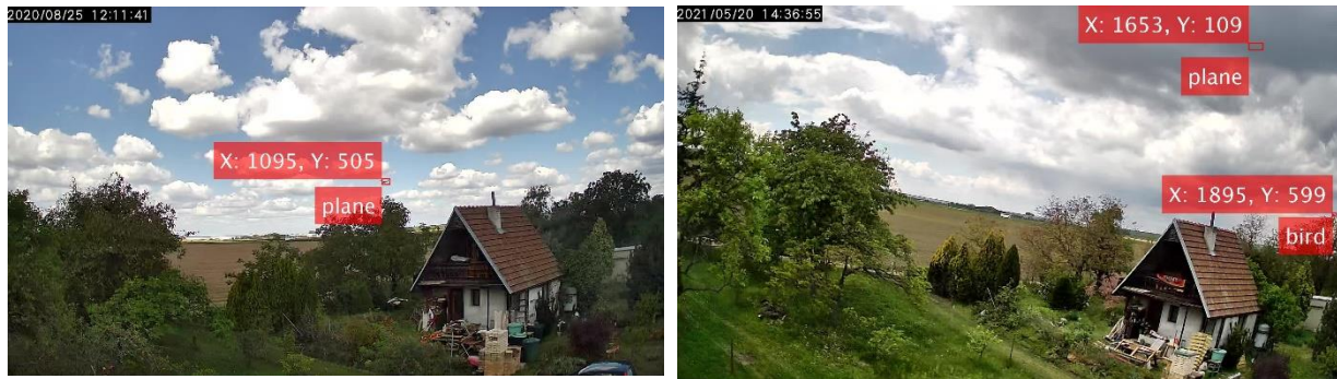
Figure 4: On the left, an example of correct aircraft detection, with display of image coordinates and class, on the right, incorrect prediction of ‘plane’ and ‘bird’ classes when detecting the movement of clouds and branches
