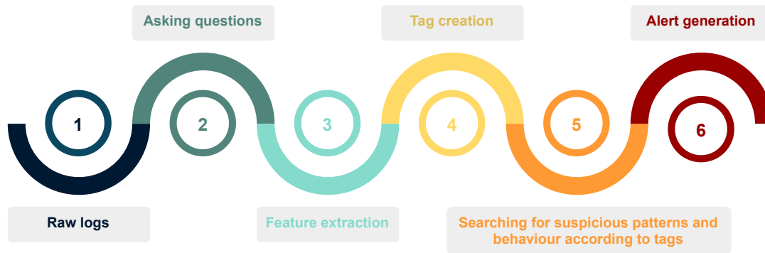
Figure 1: Work process of developed SIEM.
