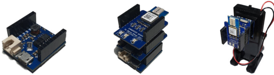
Figure 3: Battery shield, complete stack, stack with battery
