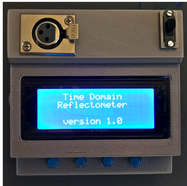
Figure 3: The first prototype of the microphone cable tester.
