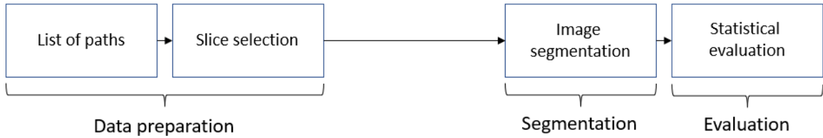
Figure 1: Block diagram of proposed workflow of full image segmentation.
