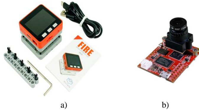
Figure 2: a) M5Stack module b) OpenMVH7 Plus camera
