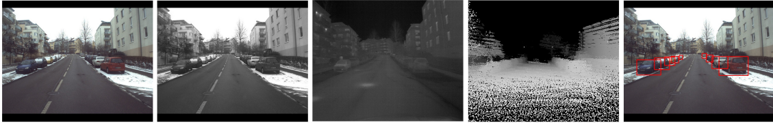
Figure 1: Tuple of annotated multi-modal data. From left, RGB image, information reduced grayscale image, thermal image, depth map image and annotations visualized on RGB image on the right. Annotations are same for all images.
