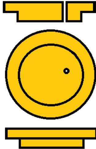
**Figure 3.** Upper electrode with a hole through which the air can escape
