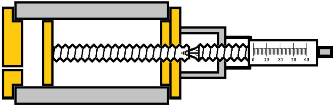
**Figure 5.** Complete assembly of the newly proposed test fixture with calliper.
