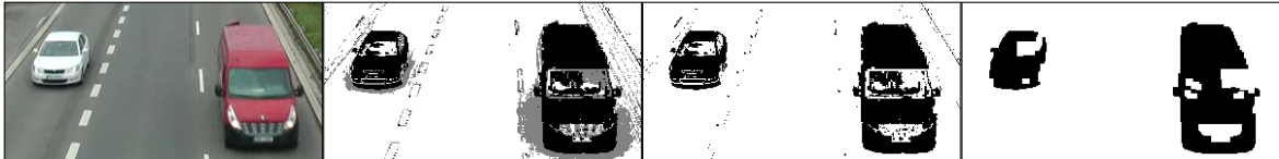
Figure 2: Process of motion detection. The leftmost image represents the original, the next one shows the detected motion with shadows which were removed in the third image. The result after the morphology opening and closing is shown in the last image.
