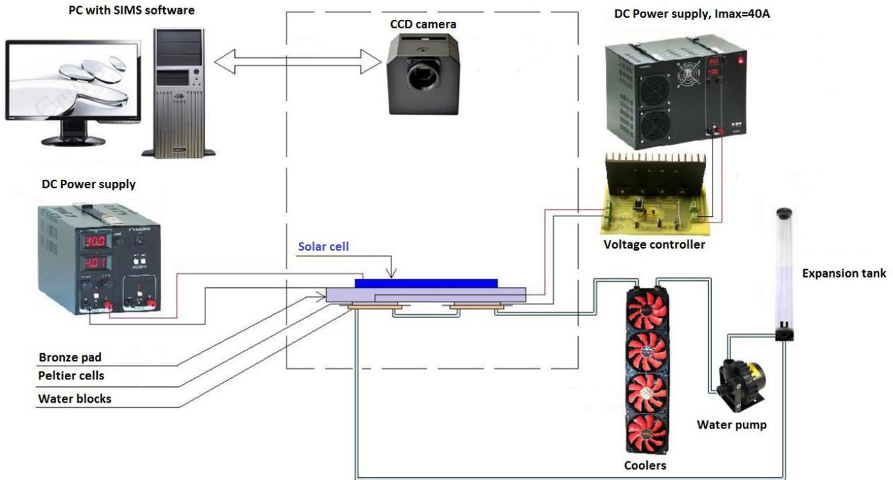
**Figure 1:** Measurement workplace of solar cells with temperature control
