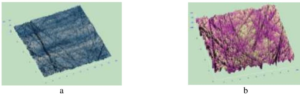
**Figure 2:** Al<sub>2</sub>O<sub>3</sub> substrate (a) before and (b) after plasma etching
