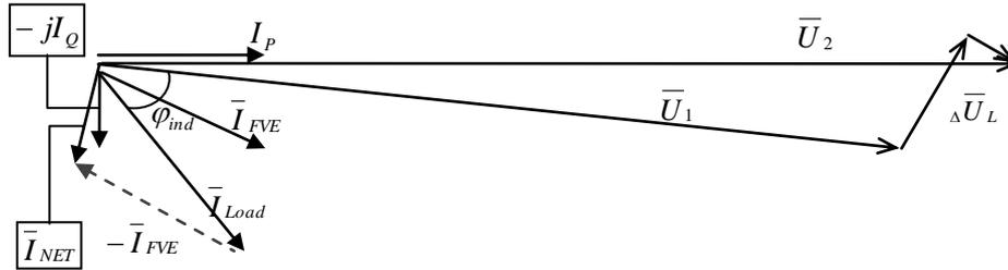
**Figure 7:** Phasor diagram of PV plant operation with capacitor – PVE supplies reactive power
