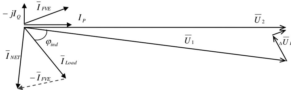
**Figure 8:** Phasor diagram of PV plant operation with reactor – PVE consumes reactive power
