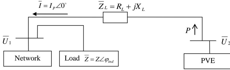
**Figure 2:** Line model for voltage growth assessment
