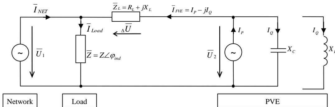
**Figure 6:** Equivalent circuit for voltage change assessment of PVE with reactive power
