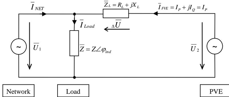
**Figure 3:** Equivalent circuit for voltage growth assessment
