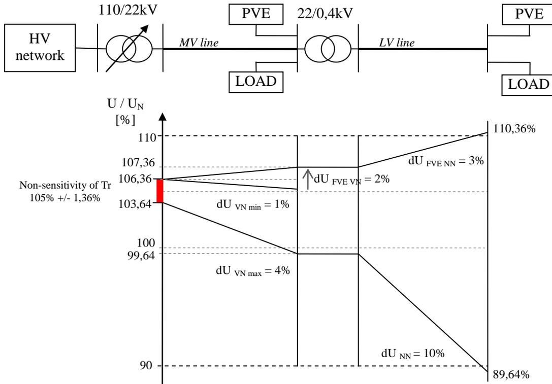
**Figure 1:** Mechanism of exceeding voltage limits due to operation of PVE [2]
