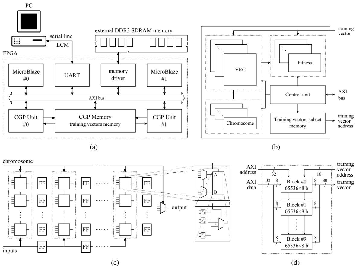
**Figure 1:** (a) Hardware platform scheme, detailed architecture of (b) CGP Unit, (c) Virtual Reconfigurable Circuit and (d) CGP Memory.
