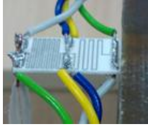
Figure 2: Probe of TDS attached to cooler.
