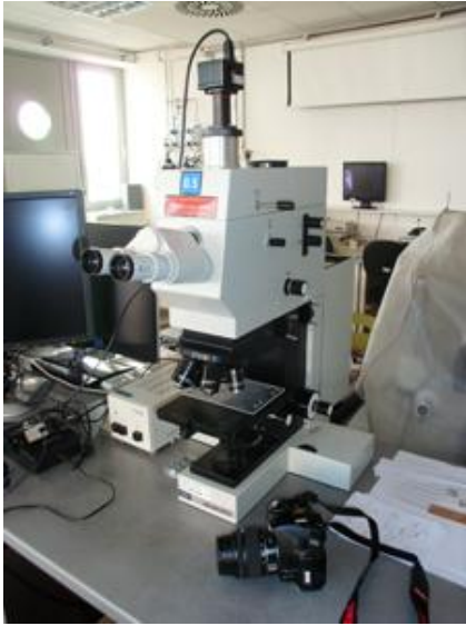
Figure 1: A digital camera placed on a microscope ocular.
