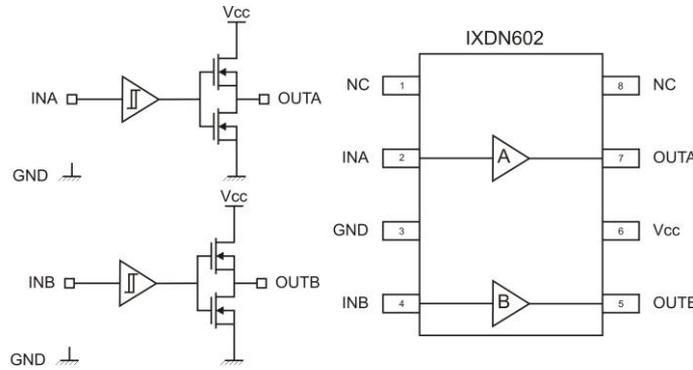
**Figure 3:** Internal structure of output stage of driver with circuit IXDN602 [taken from 5]
