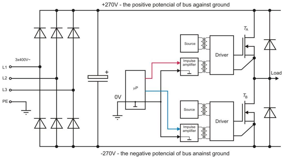
**Figure 1:** Galvanic isolation of control signals by drivers.
