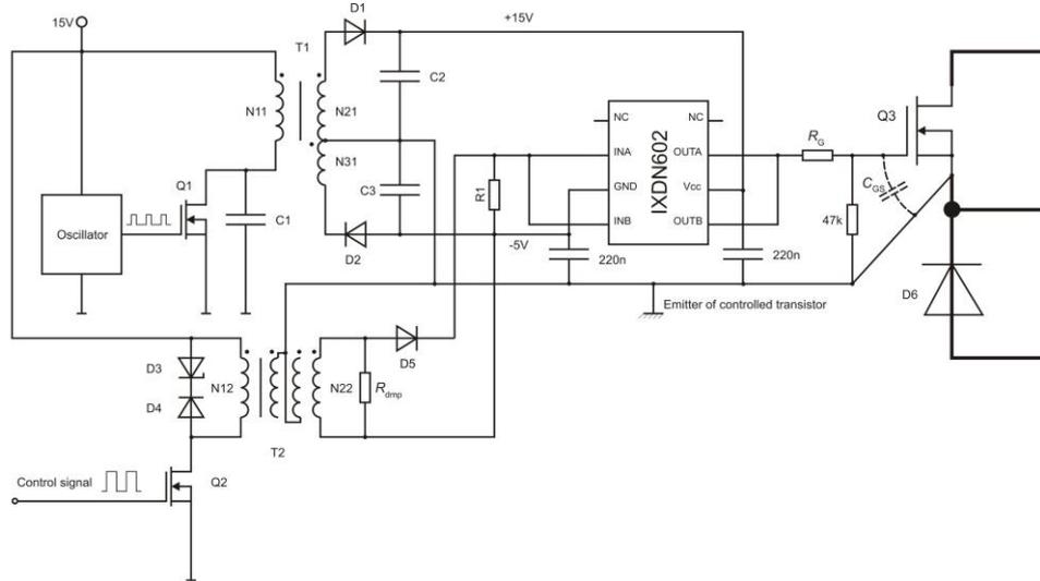
**Figure 2:** The circuit solution of driver.
