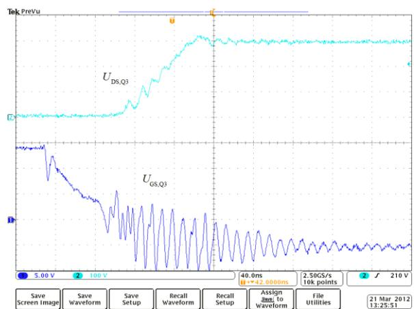
**Figure 5:** Voltage on control electrode of switching transistor  $u_{GS,Q3}$  and voltage  $u_{DS,Q3}$  for turn-off of loading transistor ( $I_D = 6A$ ,  $U_d = 300V$ )
