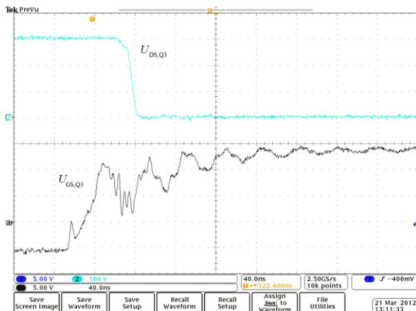
**Figure 4:** Voltage on control electrode of switching transistor  $u_{GS,Q3}$  and voltage  $u_{DS,Q3}$  for turn-on of loading transistor ( $I_D = 6A$ ,  $U_d = 300V$ )
