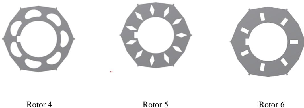
**Figure 2:** Rotor with different cooling channels shapes.
