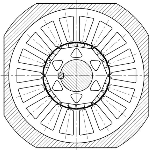
**Figure 1:** Cross section of servo motor M 718 [5].
