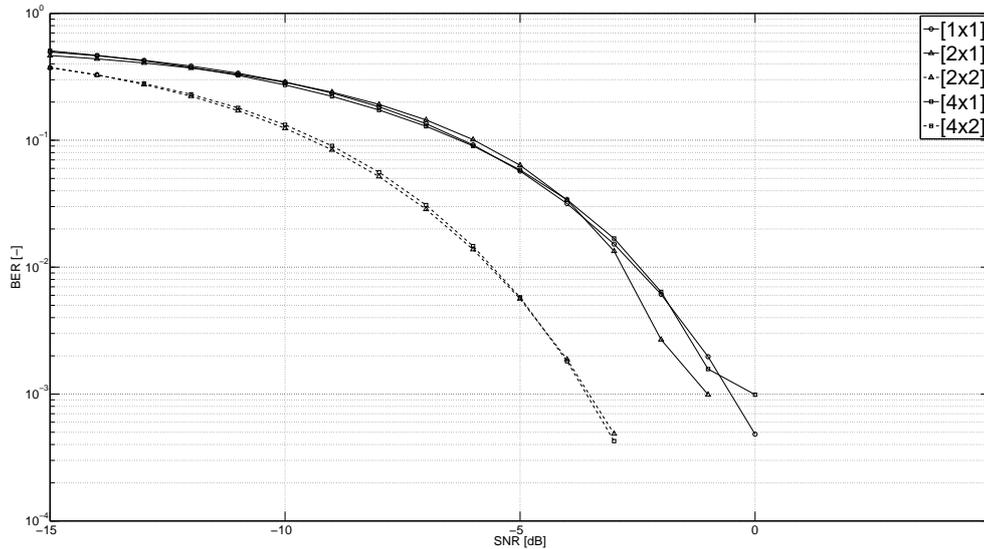
**Figure 2:** Bit error rate PCFICH in AWGN channel,  $N_{\text{subf}} = 2000$ .
