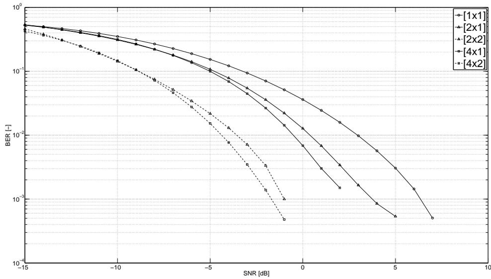
**Figure 3:** Bit error rate PCFICH in Pedestrian B channel,  $N_{\text{subf}} = 2000$ .
