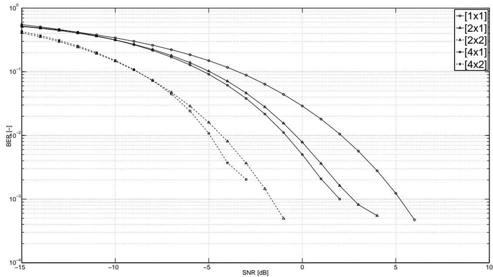
**Figure 4:** Bit error rate PCFICH in Typical Urban channel,  $N_{\text{subf}} = 2000$ .
