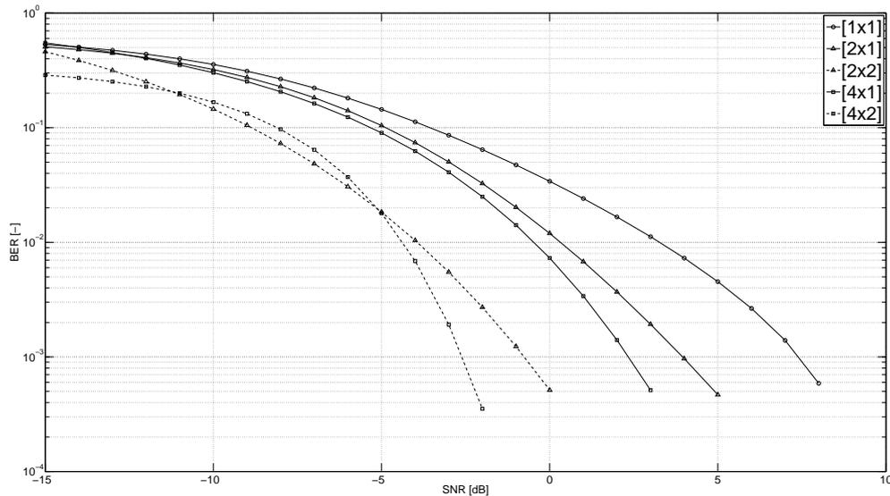
**Figure 5:** Bit error rate PCFICH in Vehicular A channel,  $N_{\text{subf}} = 2000$ .
