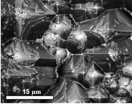
**Figure 1:** The solar cell surface topography image - pyramidal texture (typical sample)
