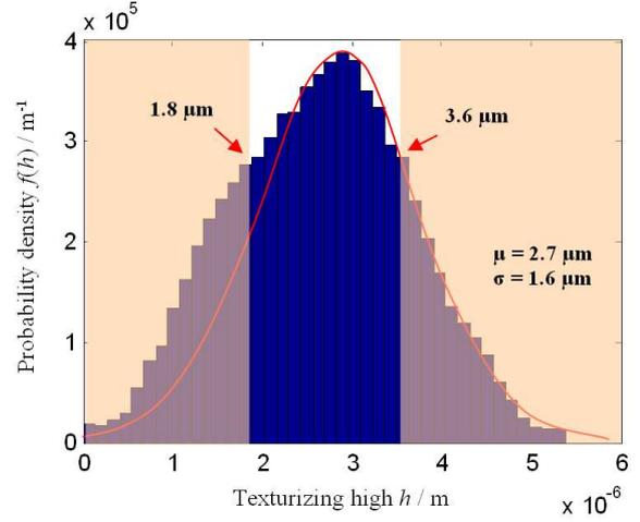
**Figure 2:** Probability density distribution of the solar cell surface high, sample labeled Q1
