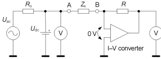
**Figure 3:** C-V characteristics measurement set-up principle of operation,  $Z_x$  is impedance of sample
