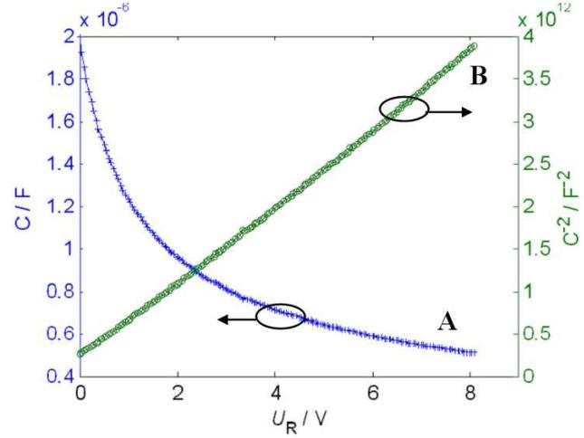
**Figure 4:** Experimental characteristics  $C = f(U_R)$  and  $C^2 = f(U_R)$  of sample 25A\_1 in dark environment,  $T = 27 \text{ }^\circ\text{C}$
