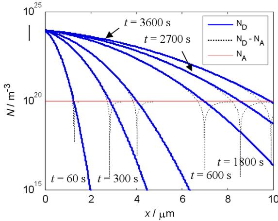
**Figure 5:** Diffusion process simulation,  $N_0 = 10^{24} \text{ m}^{-3}$ ,  $N_a = 10^{20} \text{ m}^{-3}$ ,  $D = 9 \cdot 10^{-16} \text{ m}^2 \text{ s}^{-1}$
