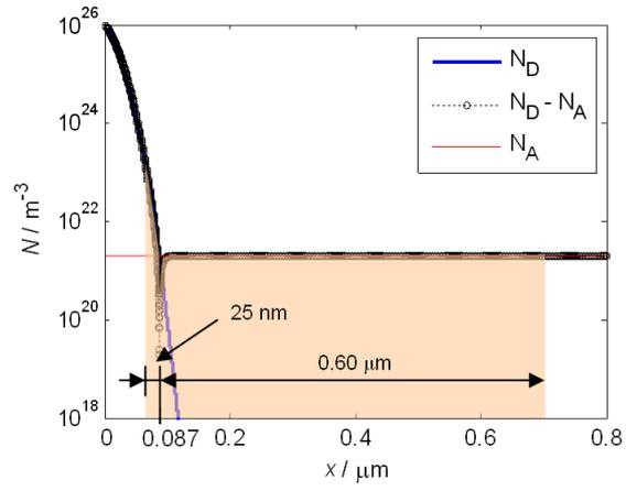
**Figure 6:** Solar cell pn junction simulation, substrate acceptor con.  $N_a = 1.1 \cdot 10^{21} \text{ m}^{-3}$ ,  $N_0 = 10^{26} \text{ m}^{-3}$ ,  $D = 5.8 \cdot 10^{-20} \text{ m}^2 \text{ s}^{-1}$ ,  $t = 3600 \text{ s}$
