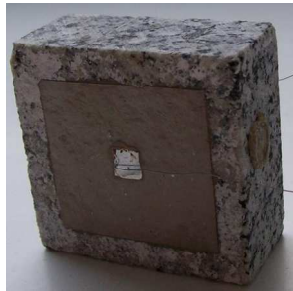
Fig. 3: The rock sample of granite. We can see electric contact on the sample fixed by DiAg paste
