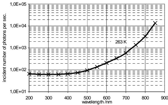
**Figure 3** Detection limit as a function of wavelength; PMT temperature  $T = 263$  K
