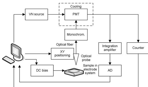
**Figure 1** Computer controlled measurement system for low radiant flux detection using PC mode and analog measurement mode
