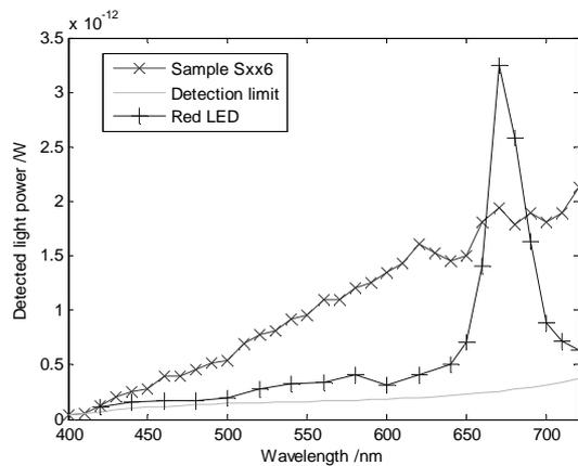
**Figure 5** Measurement of light emission spectra of sample Sxx6 and red LED radiation spectrum using analog measurement mode; PMT temperature  $T = 263$  K
