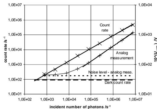
**Figure 2** Linearity of count rate in PC mode and measured voltage for analog mode, excitation wavelength  $\lambda = 650 \text{ nm}$ ; PMT temperature  $T = 263 \text{ K}$
