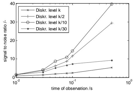
**Figure 4** SNR as a function of observation time; PMT temperature  $T = 263$  K
