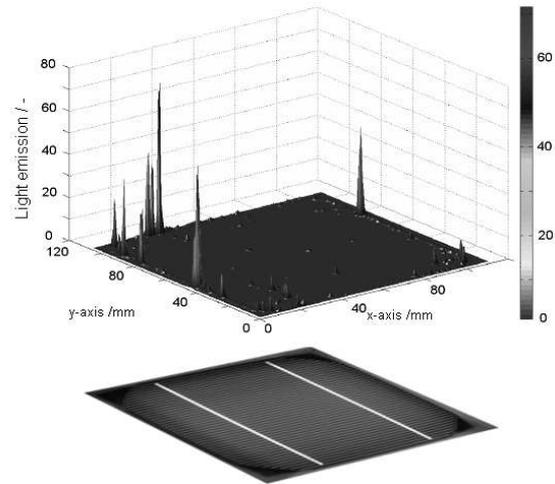
**Figure 6** Localization of imperfection areas of solar cell sample using reverse bias light emission.
