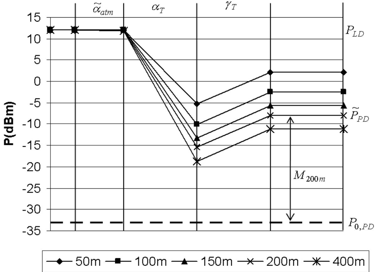
**Fig. 2:** Link budget of TereScope 700/G for different distances and  $\tilde{\alpha}_{l,atm} = 0.5 \text{ dB/km}$
