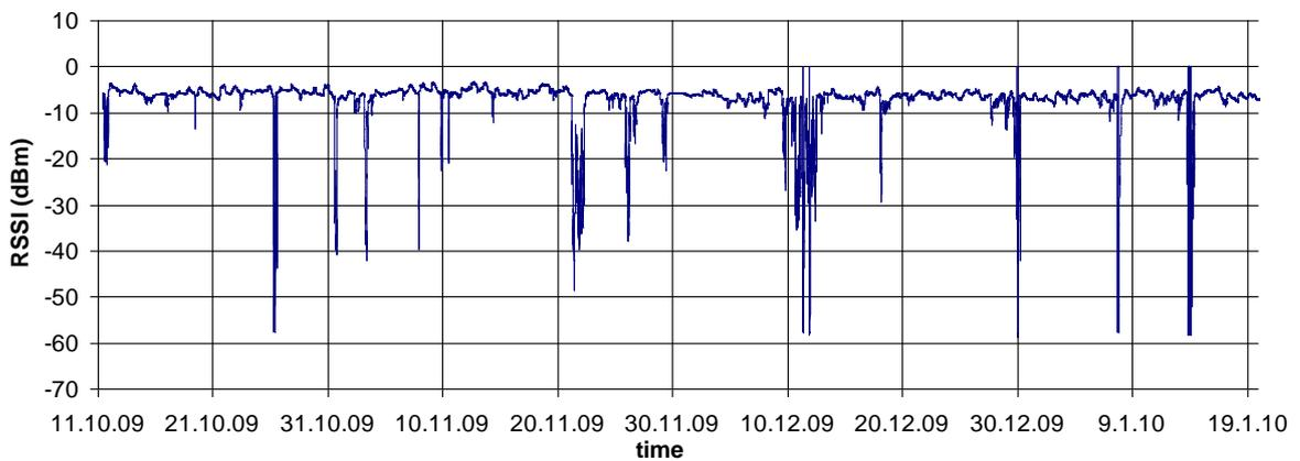
**Fig. 4:** RSSI of test FSO data link
