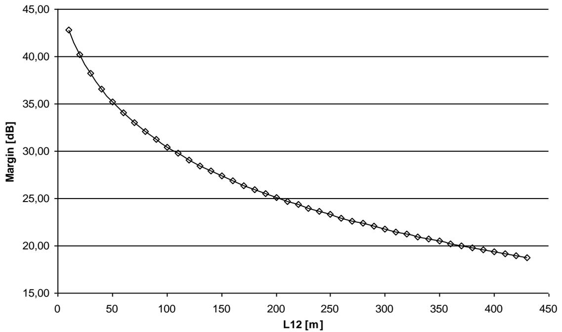
**Fig. 3:** Margin of TereScope 700/G for different distances and  $\tilde{\alpha}_{l,atm} = 0.5 \text{ dB/km}$
