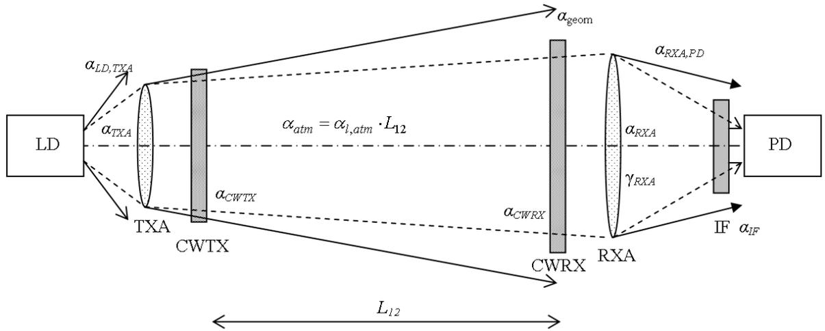
**Fig. 1:** Simplified model of FSO data link.
