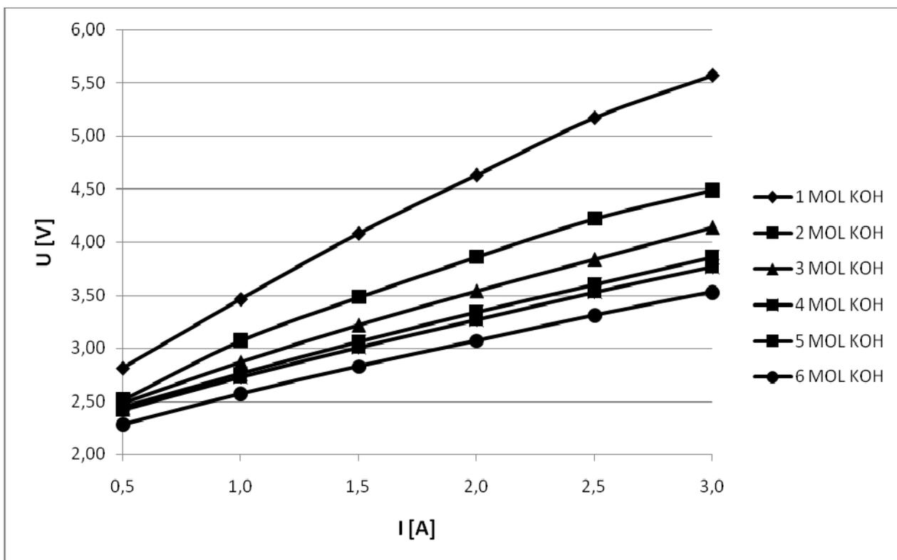
**Fig. 1** - Measurements on electrolyzer with different KOH solutions
