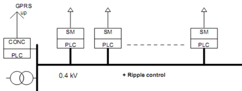
**Figure 3:** Smart meters with PLC communication. [7]
