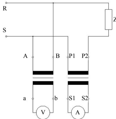
**Figure 1:** Connection of instrument transformers to the network.
