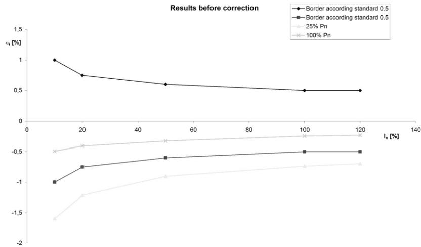
**Figure 2:** Result according of calculation without correction
