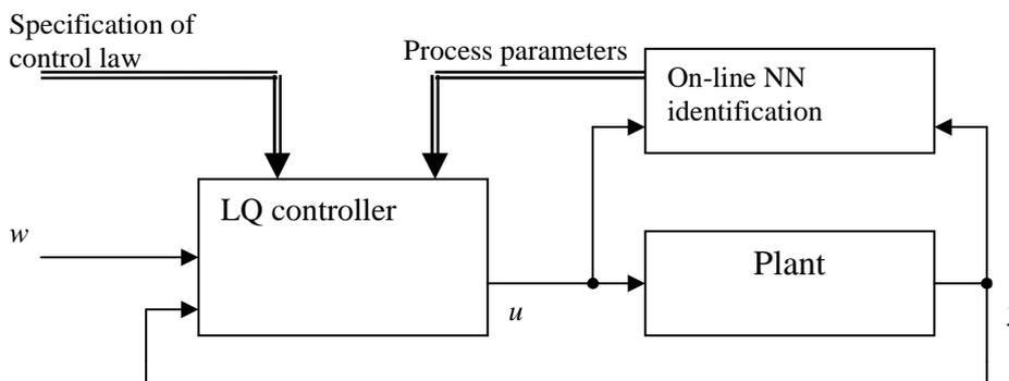
**Figure 1:** Architecture of self-tuning LQ controller.
