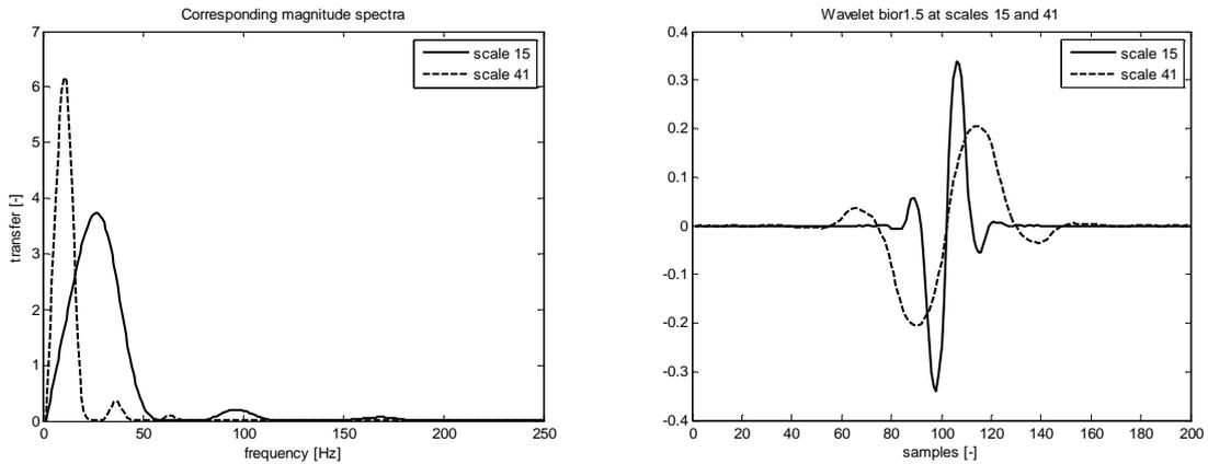
**Figure 1:** Corresponding magnitude spectra (left) and wavelets *bior1.5* (right) at the specific scales 15 and 41.
