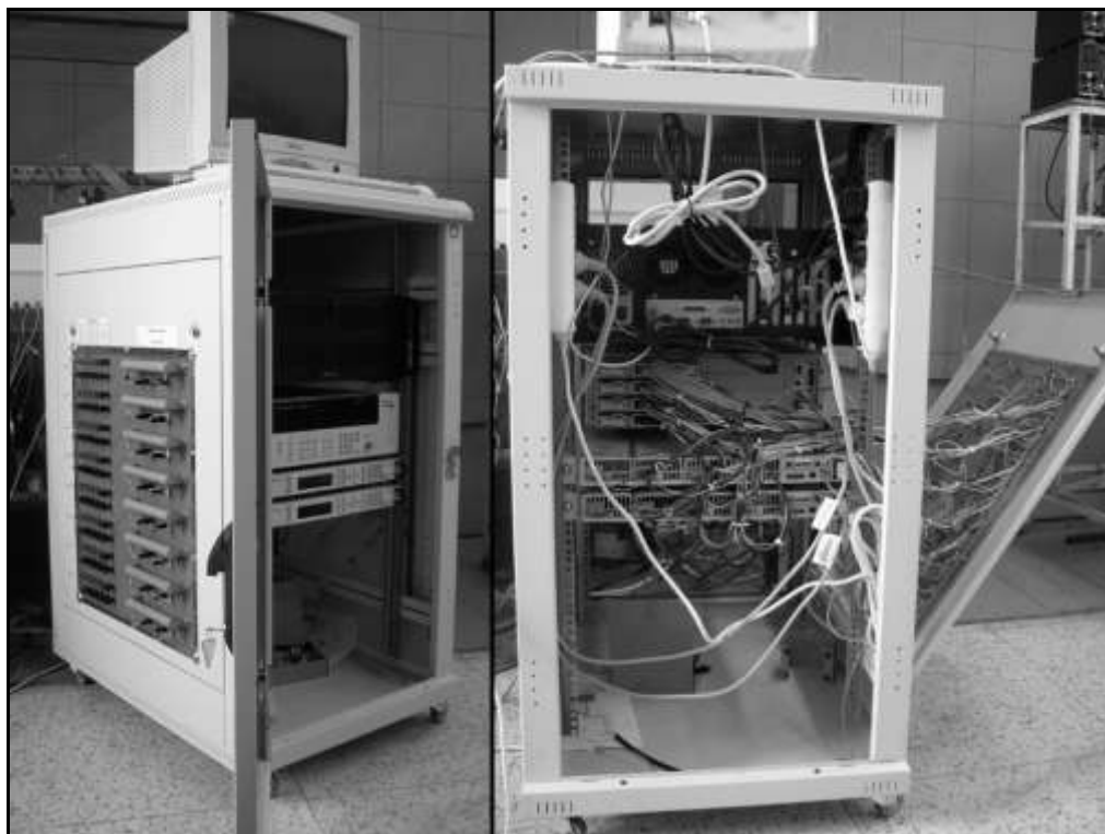
Fig. 2: The measuring apparatus for the automatic laboratory cells cycling.
