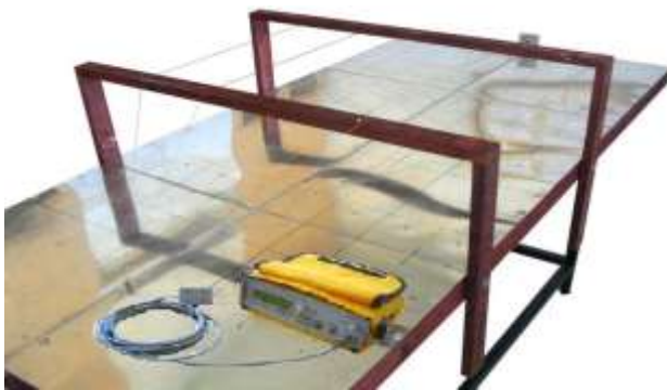
Fig. 5: Made model of simulator and shielded loop with selective microvoltmeter
