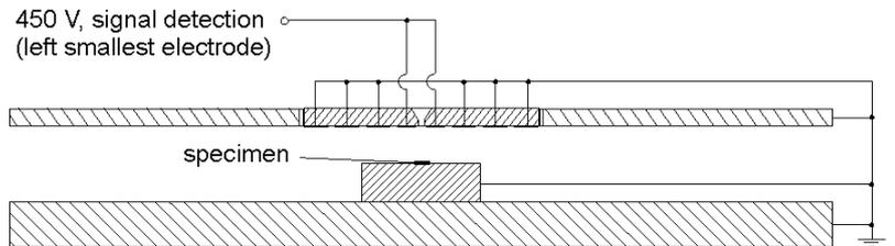
**Fig. 4:** Signal detection with halved segmental ionization detector by electrodes  $A_L + A_R$  at voltage of 450 V; all other electrodes and specimen grounded; distance between electrodes and specimen 3 mm
