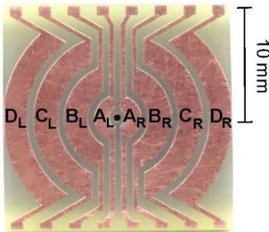
**Fig. 3:** Halved segmental ionization detector
