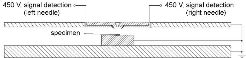
**Fig. 2:** Signal detection with needle ionization detector by left or right needle electrode at voltage of 450 V; distance between electrodes and specimen 2 mm; specimen grounded
