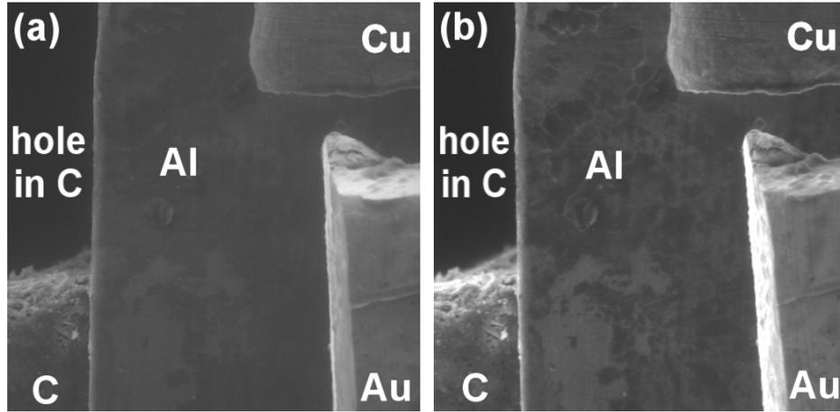
**Fig. 6:** Material and topographic contrasts; specimen consisting of hole in carbon, carbon, aluminium foil, cuprum foil and gold foil; water vapors environment 700 Pa, mag. 700x; (a) needle ionization detector, detection by left needle electrode at voltage of 450 V; (b) halved segmental ionization detector, detection by electrodes  $A_L+A_R$  at voltage of 450 V; all other electrodes grounded; 10 times higher probe current in case of (a) then in case of (b)
