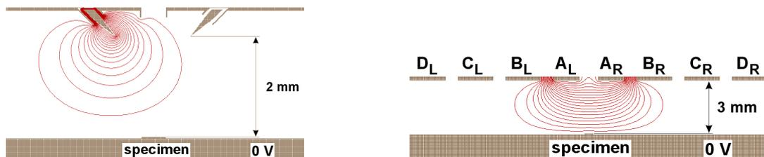
**Fig. 7:** Equipotent lines for needle ionization detector (left) and halved segmental ionization detector (right); voltage of 450 V on left needle electrode; voltage of 450 V on electrodes  $A_L+A_R$ ; other electrodes and specimen grounded; equipotent lines by 22.5 V
