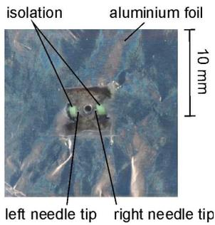
**Fig. 1:** Needle ionization detector; aluminium foil grounded
