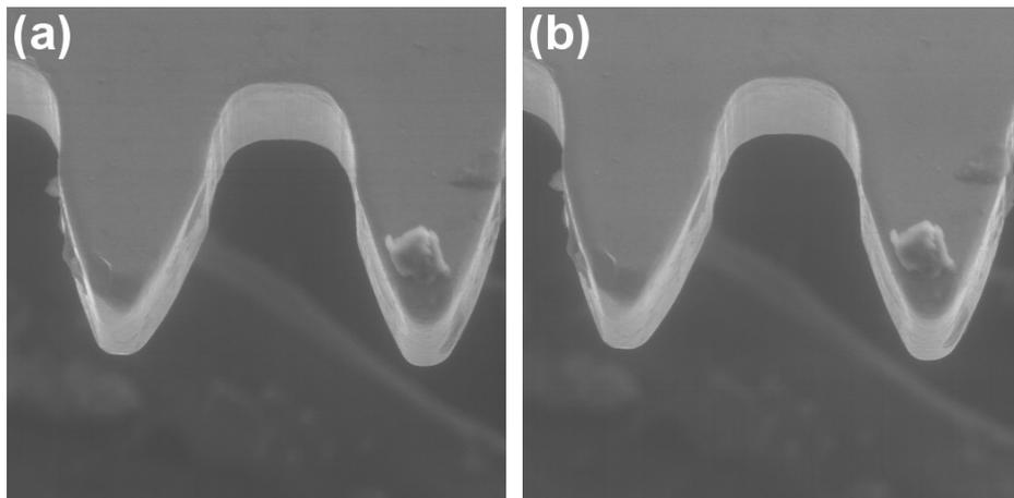
**Fig. 5:** Signal detection by needle ionization detector by left (a) and right (b) needle electrode at voltage of 450 V; brass toothed wheel, water vapors environment 700 Pa, magnification 500x
