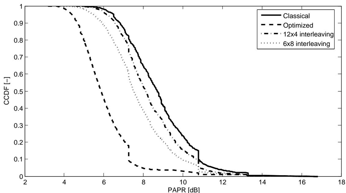
Figure 5: Comparison of optimized sequence and matrix interleavers
