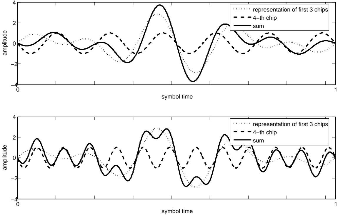
Figure 2: The idea of PAPR reduction. The chip sequence [1 -1 1 -1] is used. First 3 chips are modulated on 3. 4. and 5. subcarrier. 4. chip is modulated on 6. subcarrier in upper figure and on 12. subcarrier in lower.
