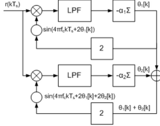
**Fig. 1:** Dual PLL system used in model.
