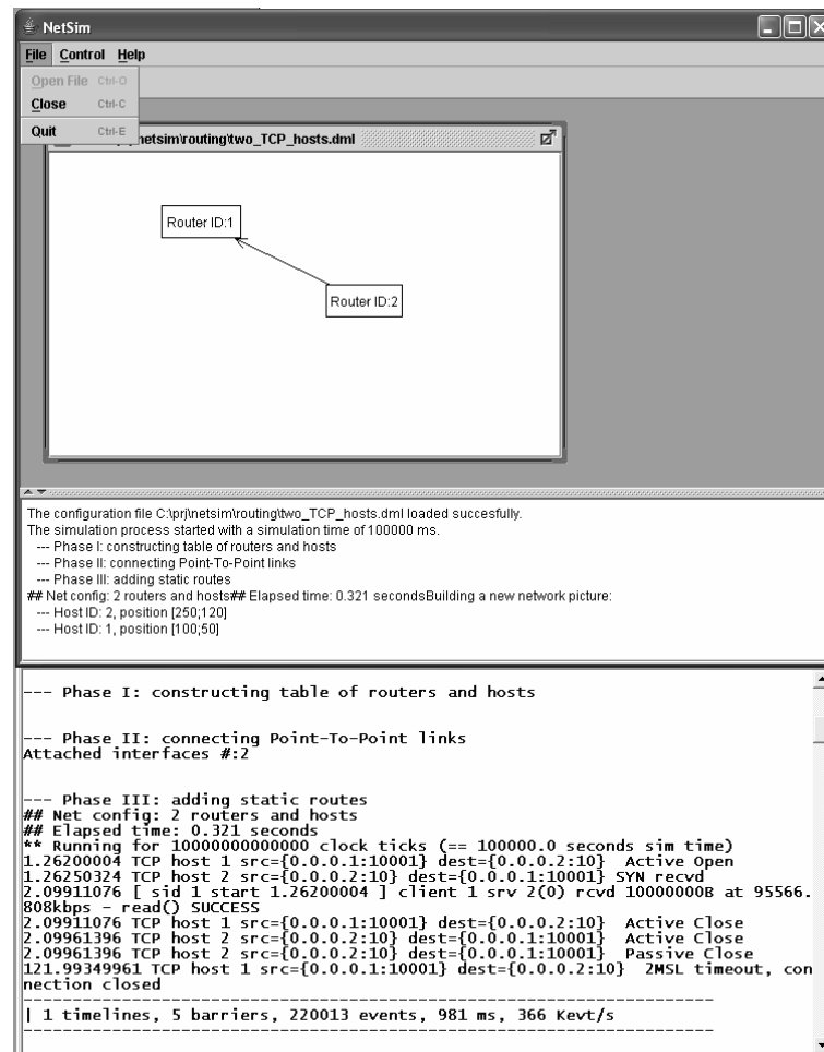
Fig. 1: The NetSim application window shows results of a simple SSFNet client-server simulation.
