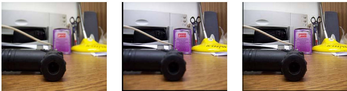
Fig. 4: On the left is foreground focused image, in the middle is background focused image and on the right is the image fused using proposed algorithm.
