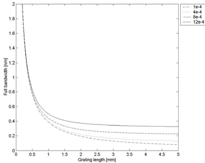
**Fig. 4:** Full bandwidth as function of grating length, calculated for SG682 fiber, parameter  $\delta n$
