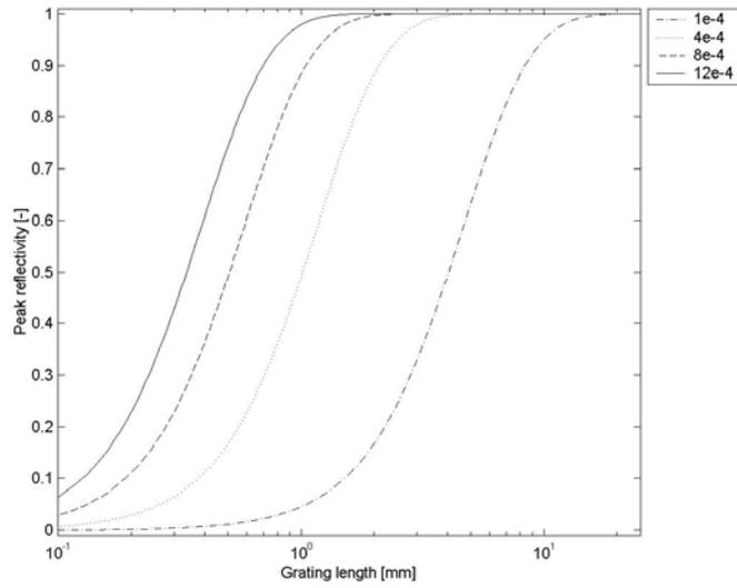
**Fig. 3:** Peak reflectivity as function of grating length, calculated for SG682 fiber, parameter  $\delta n$
