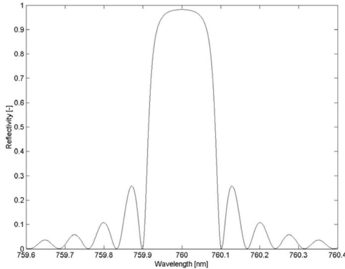
**Fig. 2:** Reflectivity against wavelength, calculated for grating length 2.5mm and  $\delta n = 5 \times 10^{-4}$  in SG682 fiber
