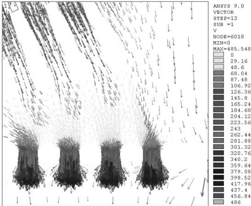
Figure 2: Visualisation of velocities using vector field in a side view
