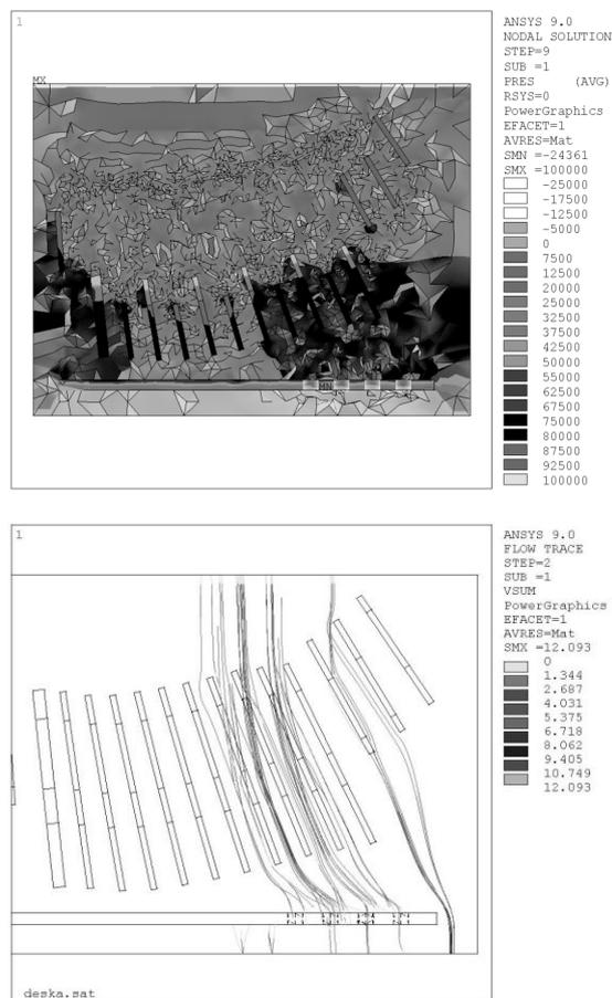
Figure 3: Visualisation of pressure distribution in lengthwise section (left) and streamlines (right)
