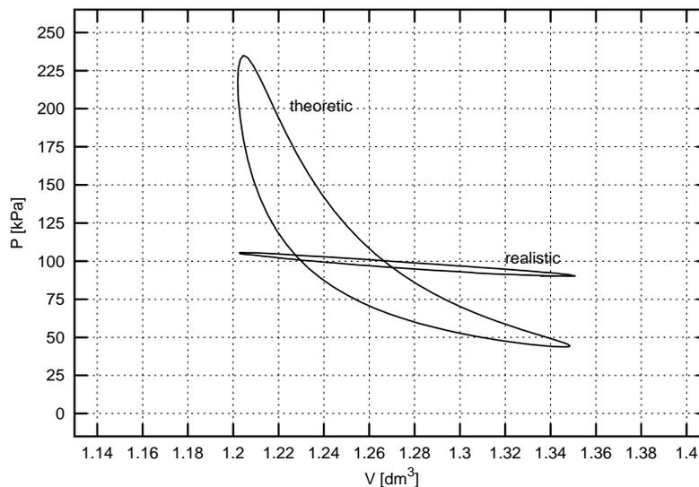
Figure 2: p - V diagrams of theoretic and realistic engine.
