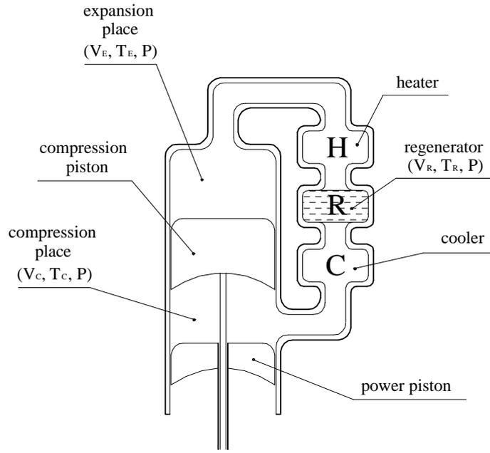
Figure 1: Construction of  $\beta$  engine modification.
