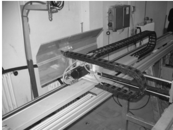
Fig. 1: Two-axes support and tested nozzle (upper left corner)
