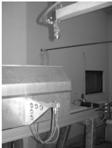
Fig. 2: Pressure sensor mounted on the shorter axis and the tested nozzle
