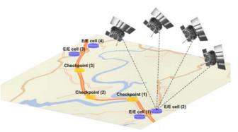
Fig. 4: Virtual Tolling System Architecture
