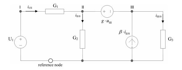
Fig. 1: An example of a linear circuit. Some variables are not drawn.
