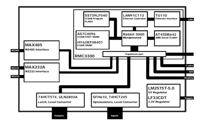
Fig. 1: OMICRON-II block diagram
