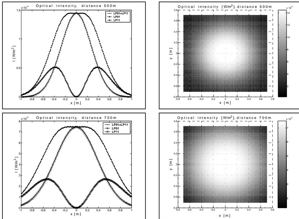
**Fig. 3:** *The distribution of the optical intensity in the plane of receiver.*
