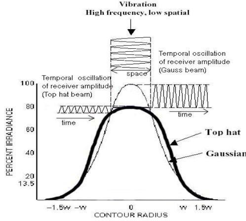
**Fig. 1:** *The impact of high frequency, low amplitude vibration on the temporal amplitude of the receiver for the Gaussian beam and the top hat beam.*
