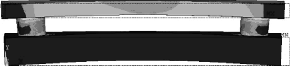
Fig. 5: Internal stresses of the structures with 0.7 mm solder high
