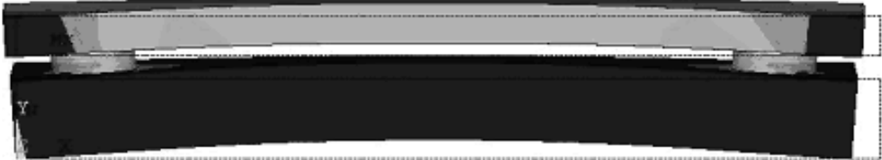
Fig. 2: Internal stresses of the structures with 0.3 mm solder high
