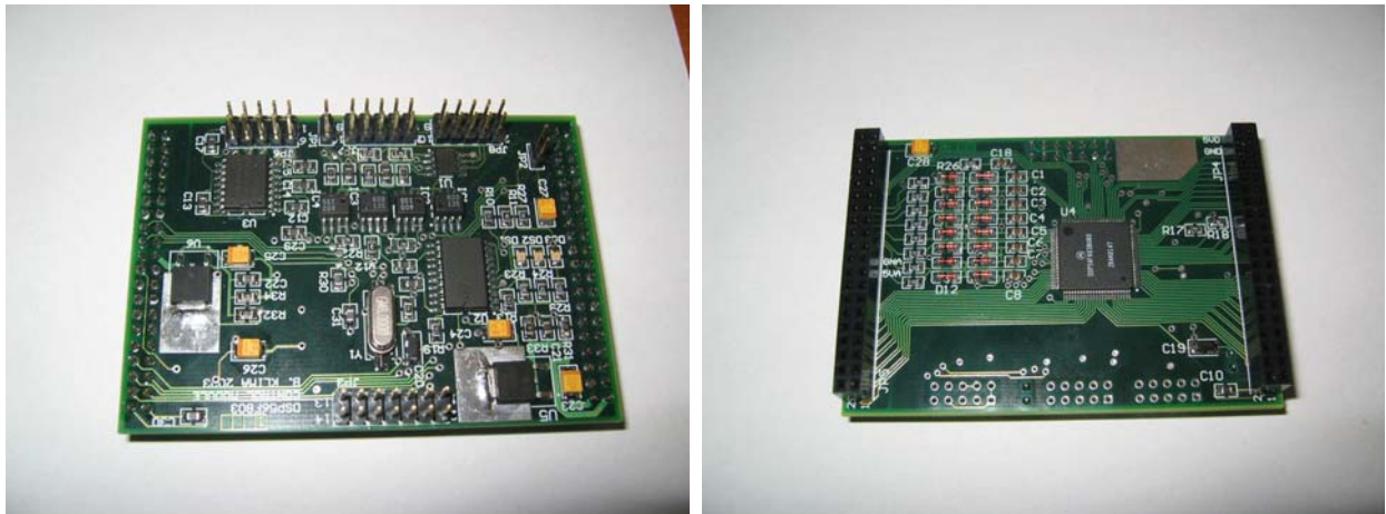
Fig. 1: Module with DSP 56F803 (on the left is top layer, on the right is bottom layer)
