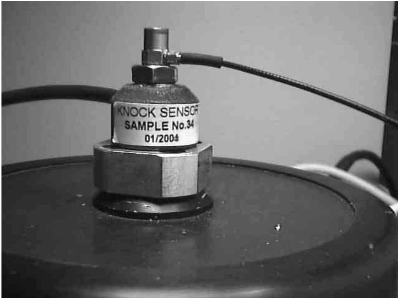
Fig. 3: Detail of gripping knock sensor to shaker and gripping reference accelerometer
