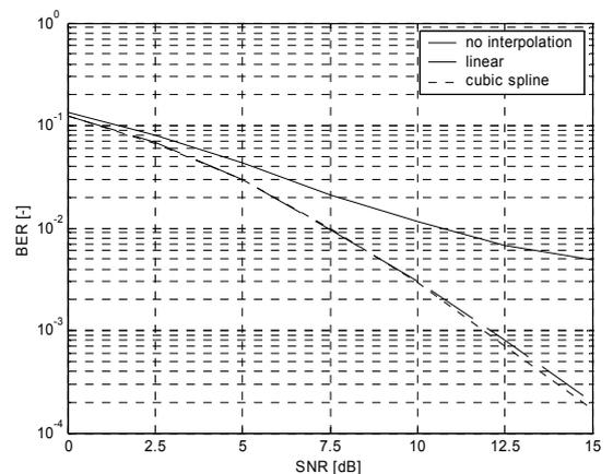
**Fig. 2:** *Uncoded BER performance for  $N = 50$  with none, linear and cubic spline interpolation*
