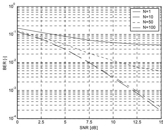
**Fig. 1:** *Uncoded BER performance for  $N = 100$  with none, linear and cubic spline interpolation.*
