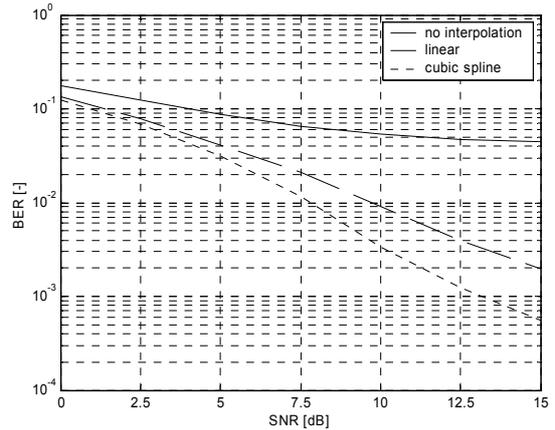
**Fig. 4:** *Uncoded BER performance for  $N = 200$  with none, linear and cubic spline interpolation*
