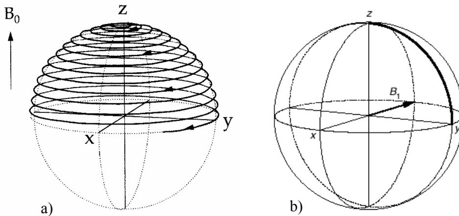
**Fig. 1:** Path of magnetization vector  $M_0$ : a) laboratory coordinate system, b) rotating coordinate system
