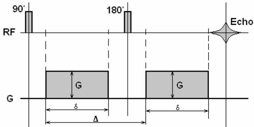
**Fig. 4:** *Pulse sequence of spin echo, with symmetrically placed diffusion gradients.*
