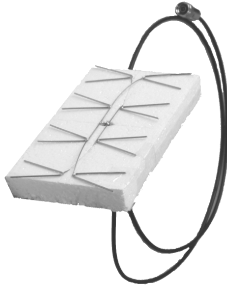
Fig. 1: 4-element stack array with reflector realization
