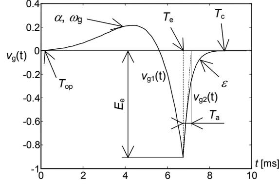
**Fig. 2:** Approximation function and the meaning of individual parameters.
