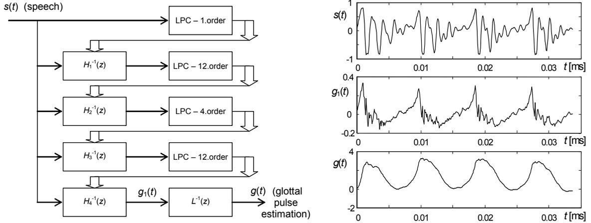
**Fig. 1:** IAIF block diagram – left, typical waveforms in block diagram – right.
