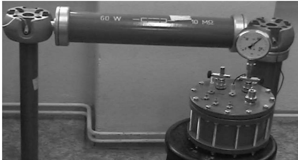
**Fig. 1:** The reaction chamber plugged into the sparking perimeter
