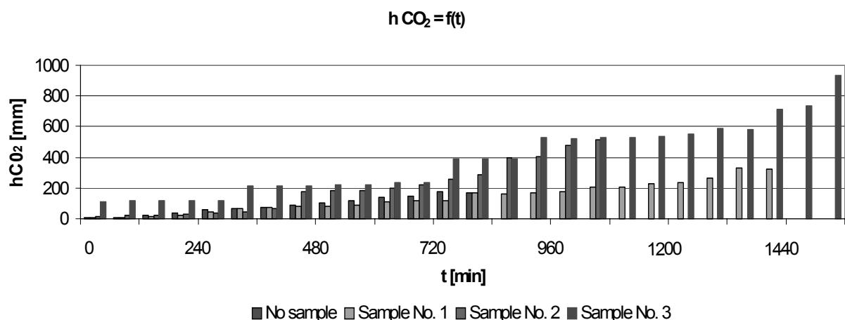
**Graph 2:** The comparing of the peaks size of the dissociative products CO<sub>2</sub> during the sparking with and without the inserted samples No. 1, 2, 3. ( $200\text{mm} \equiv 6,36 \mu\text{l}$ ).
