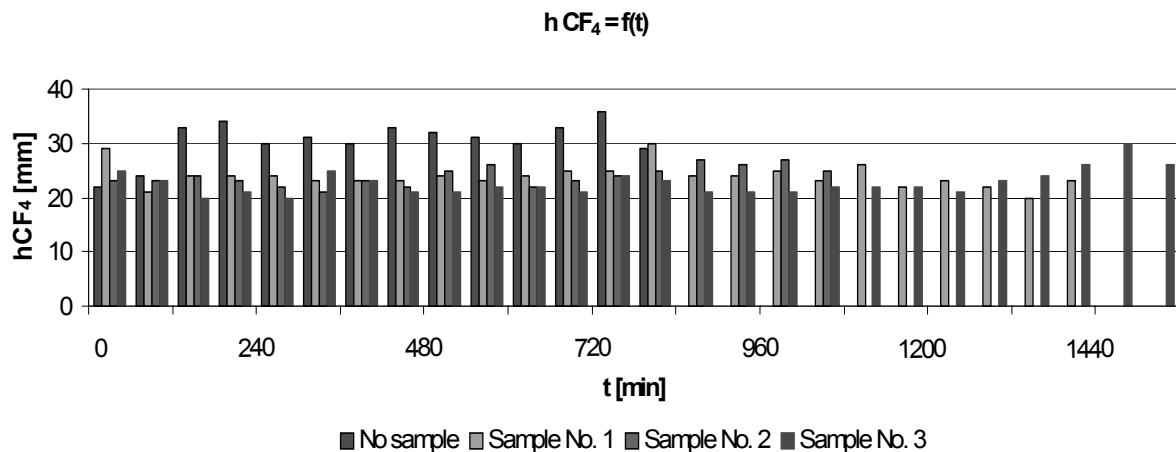
**Graph 1:** The comparission of the peaks size of the dissociative products CF<sub>4</sub> during the sparking with and without the inserted samples No. 1, 2, 3. ( $10\text{mm} \equiv 0,464 \mu\text{l}$ ).
