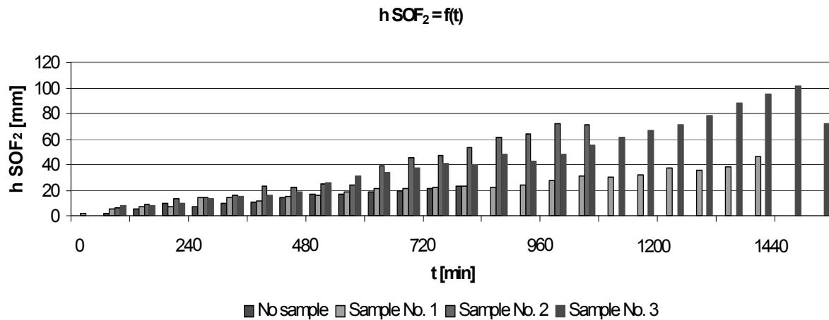
**Graph 3:** The comparing of the peaks size of the dissociative products  $\text{SOF}_2$  during the sparking with and without the inserted samples No. 1, 2, 3. ( $100\text{mm} \equiv 2,31 \mu\text{l}$ ).
