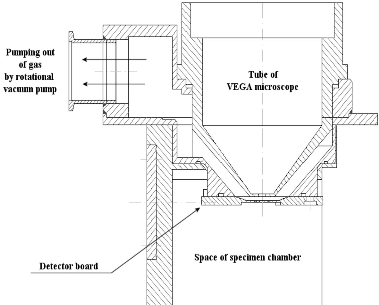
**Fig. 3:** Complete view of adapted configuration of Environmental microscope with differential pumping chamber, detector board, part of specimen chamber and part of microscope tube.
