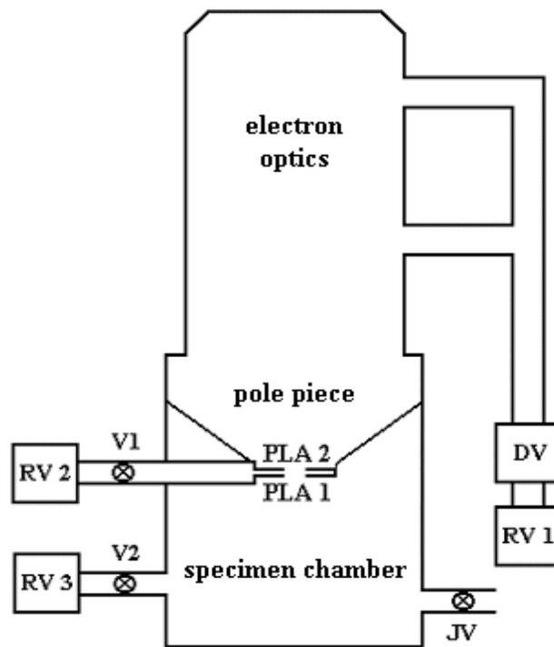
**Fig. 1:** *Schematic layout of two-stage system of differential pumping for ESEM*
