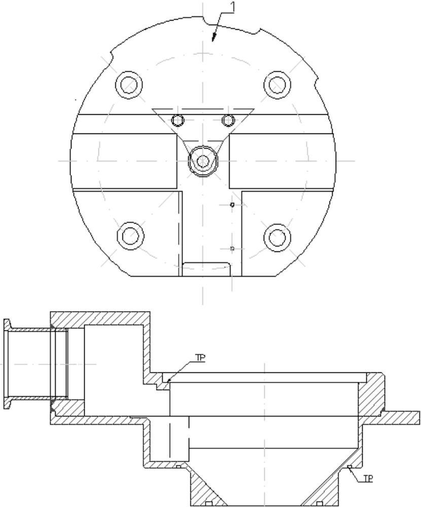
**Fig. 2:** *There is a differential pumping chamber of ESEM microscope in the bottom part of the figure and there is an upper view of detector board of differential pumping chamber in the high part.*
