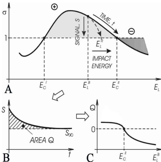
**Fig. 1:** The typical dependence of the total electron yield on the electron landing energy (A). The time dependence of the image signal (B). The dependence of area  $Q$  on the electron landing energy (C).
