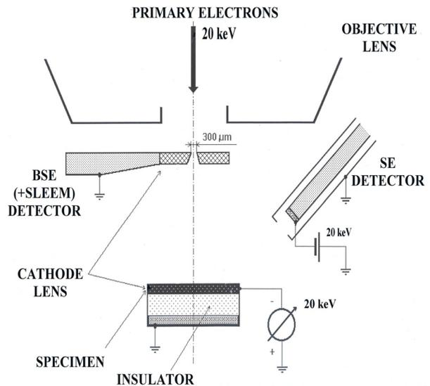
**Fig. 2:** Scheme of the specimen chamber configuration with the cathode lens.
